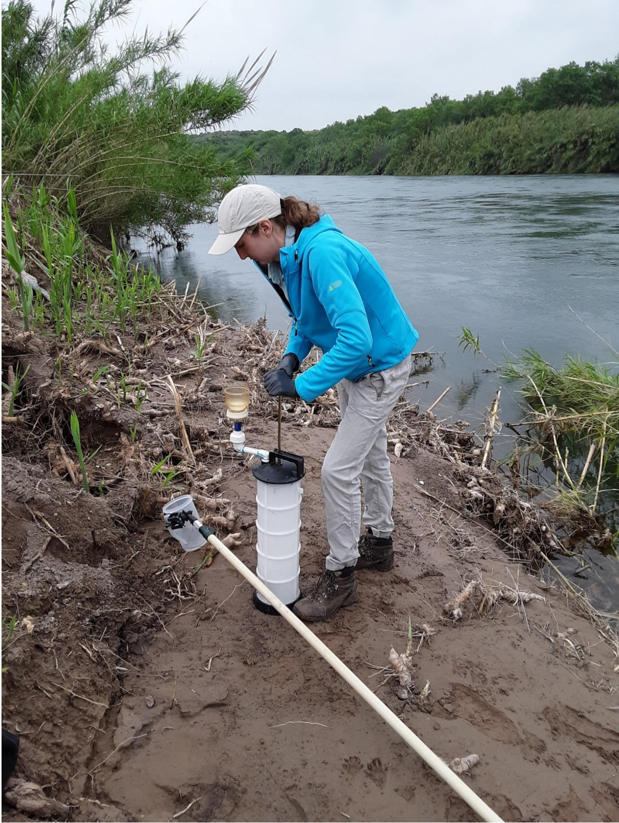
Figure 3.18. Environmental DNA (eDNA) filtering equipment, including a plastic pitcher on the end of a telescoping pole, 47-mm filter cup, and a hand-powered automotive fluid evacuator.
