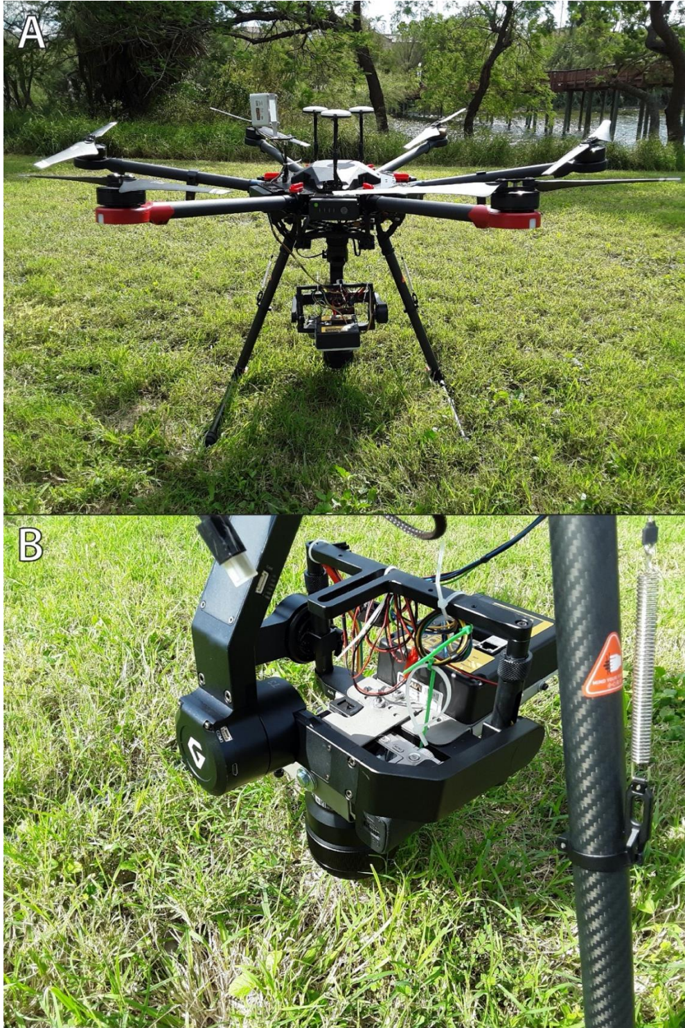
Figure 3.1. Drone and equipment used for drone surveys of Pseudemys gorzugi . A) DJI Matrice 600 Pro unmanned aerial vehicle with survey equipment attached used to survey for Pseudemys gorzugi ; B) Gremsy T-3 gimbal with the MAIA multi-spectrometer and digital camera attached. This configuration ensured equal weight distribution to assist in keeping the cameras level during flight.
